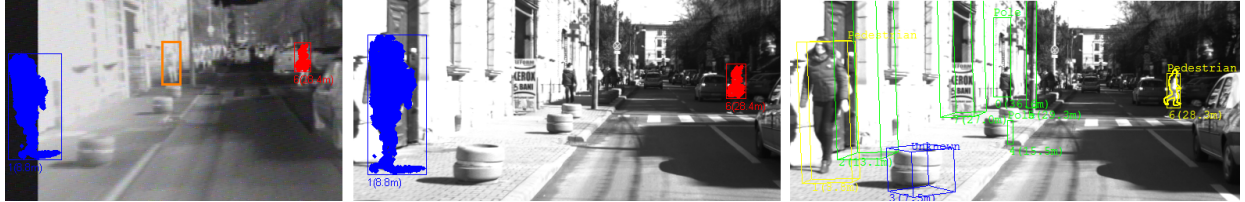
(b) Dynamic scene left - far IR image, middle - grayscale image, right - 3D hypotheses from the stereo sensor
